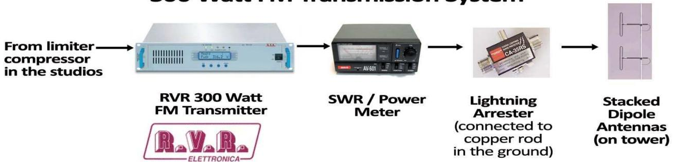
In this system, the audio signal from the studios is fed into the **transmitter**, which converts it into a radio frequency signal, and amplifies the signal to 300 Watts. This is fed into the **SWR/Power Meter**, to monitor the power and efficiency of the system. The signal then passes through a **lightning arrester**, which is connected to the earth via a copper grounding cable and 4' copper rod. From there the signal is sent to the **antenna**, to be broadcast to the surrounding area.
